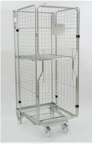
**Technical data:** the stability of construction is provided by closed profiles, nets made of steel bars, bottom with wheels (2 fixed wheels, 2 swivel wheels with brakes), bottom shelf is reinforced with flat bars. Container has front door which can be closed creating the front wall of the container. The upper shelf is folded. The construction of container allows for its folding and nesting of folding containers.
