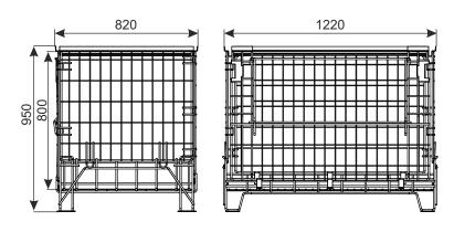
This pallet container is a full value container, making it possible to store and transport loose goods, without using euro pallets. It allows for stacking up to three containers (pallet container and the pallet) and reducing to 1/4th the warehouse floor space necessary to store the same quantity of goods. Metal feet allow the container to be lifted up by a fork-lift and also facilitate cleanliness in the warehouse.
